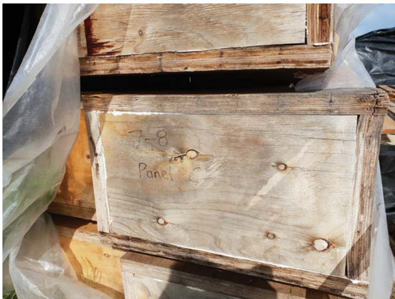
Figure 6. Panels damaged by prolonged exposure to moisture in storage.
