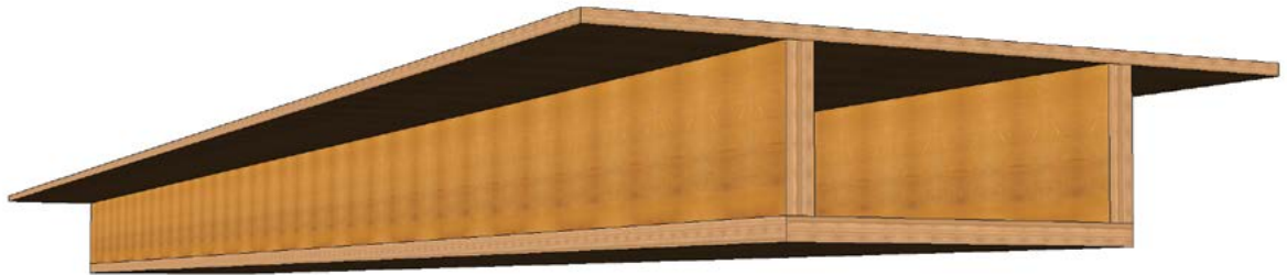
Example of a boxed flooring cassette panel.
